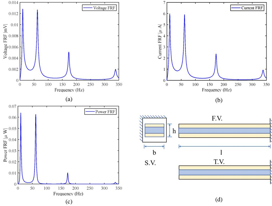
Figure 14: Analytically calculated (a) Voltage (b) Current (c) Power plots for cantilever bimorph piezoelectric energy harvester subjected to harmonic base excitation. (d) Schematic representation of cantilever bimorph PZEH.
