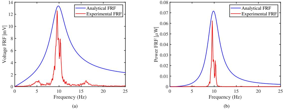
Figure 16: Topological metamaterial lattice with soft-soft ( $k_2 - k_2$ ) spring arrangement attached at the adjacent sides of interface mass along with the piezobeam attached to it for voltage and power measurement showing peak at 9.56 Hz (a) Comparison between experimental and analytical Voltage FRF (b) Comparison between experimental and analytical Power FRF.
