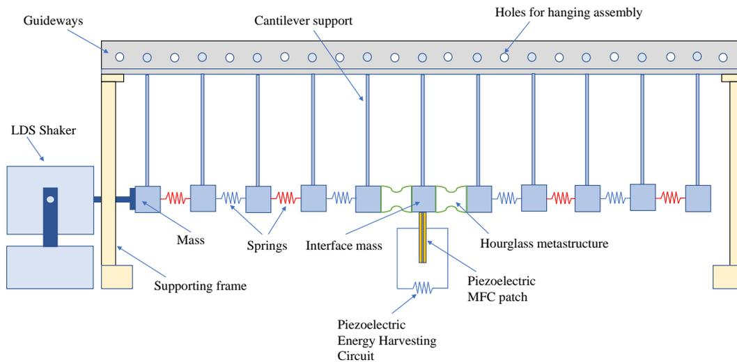
Figure 9: Conceptual schematic diagram of topological metamaterial lattice with hourglass mounted at the adjacent sides of the interface mass along with integrated piezoelectric energy harvesting circuit.
