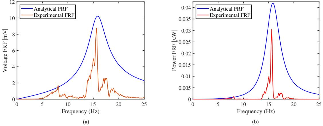
Figure 21: Modified topological lattice with ( $k_3 - k_3$ ) auxetic hourglass arrangement at adjacent sides of interface mass having stiffness parameter  $\chi \approx 50$  along with the piezobeam attached to the interface mass for voltage and power measurement showing peak at 15.63 Hz (a) Comparison between experimental and analytical Voltage FRF (b) Comparison between experimental and analytical Power FRF.
