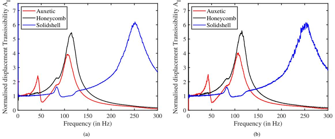
Figure 7: 3D Hourglass printed samples dynamically tested using LDS shaker with LDV data acquisition system having gain (a)  $g=1$  and (b)  $g=1.6$  upto 300 Hz.
