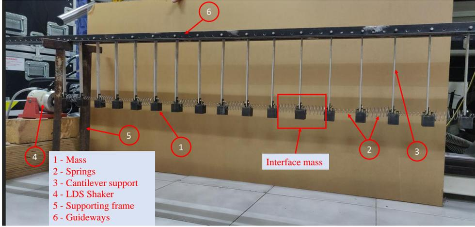
Figure 10: Experimental setup of topological metamaterial lattice with hard-hard springs arrangement at adjacent sides of interface mass i.e.  $k_1 - k_1$  to demonstrate interface mode
