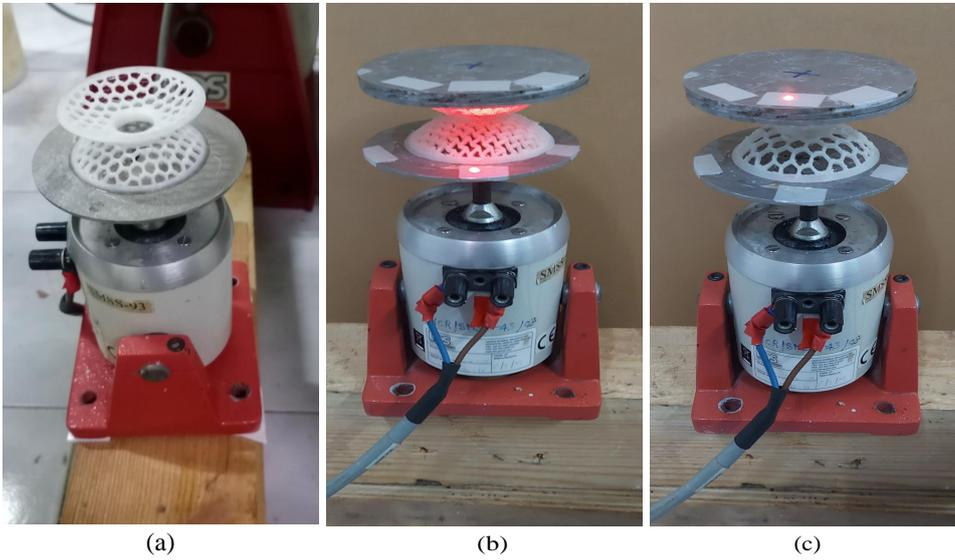
Figure 6: (a), (b) and (c) shows dynamic testing of hourglass sample using LDS shaker upto frequency range of 300 Hz with the dead weight of 100 gm mounted at the top of hourglass sample with LDV laser beam incident.
