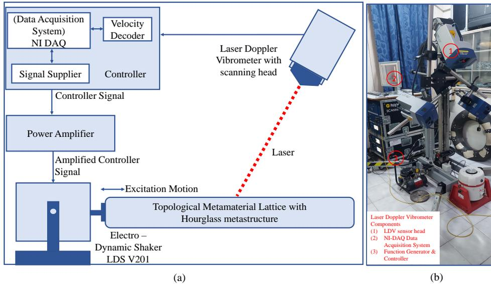
Figure 8: (a) Schematic diagram of the experimental setup with topological metamaterial lattice along with interface mode (b) Laser Doppler Vibrometer
