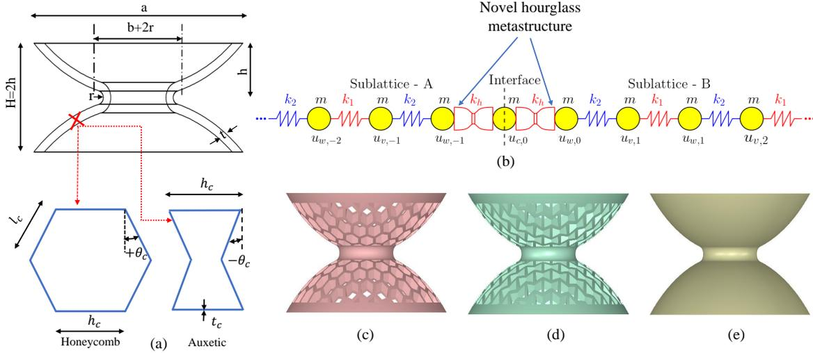
Figure 1: (a) Details of geometric specifications of hourglass lattice metastructure along with the honeycomb and auxetic cellular configurations and their dimensions. (b) Schematic representation of a novel 1D periodic spring-mass system with the introduction of hourglass metastructure at the interface junction to break the inversion symmetry. (c, d, e) Representation of homogeneous type hourglass lattice metastructure with the honeycomb, auxetic and solid shell configurations.
