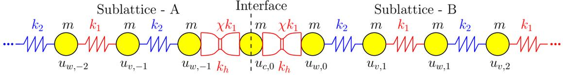
Figure 17: 1D topological metamaterial lattice having diatomic unit cells comprising identical masses  $m$  and inversion symmetry broken at the interface with hourglass metastructure having stiffness  $k_h = \chi k_1$  while the remaining lattice is connected with the linear springs having stiffness  $k_1$  and  $k_2$ , where  $k_1 = k(1 + \gamma)$ ,  $k_2 = k(1 - \gamma)$ ,  $\gamma = -0.4$ .
