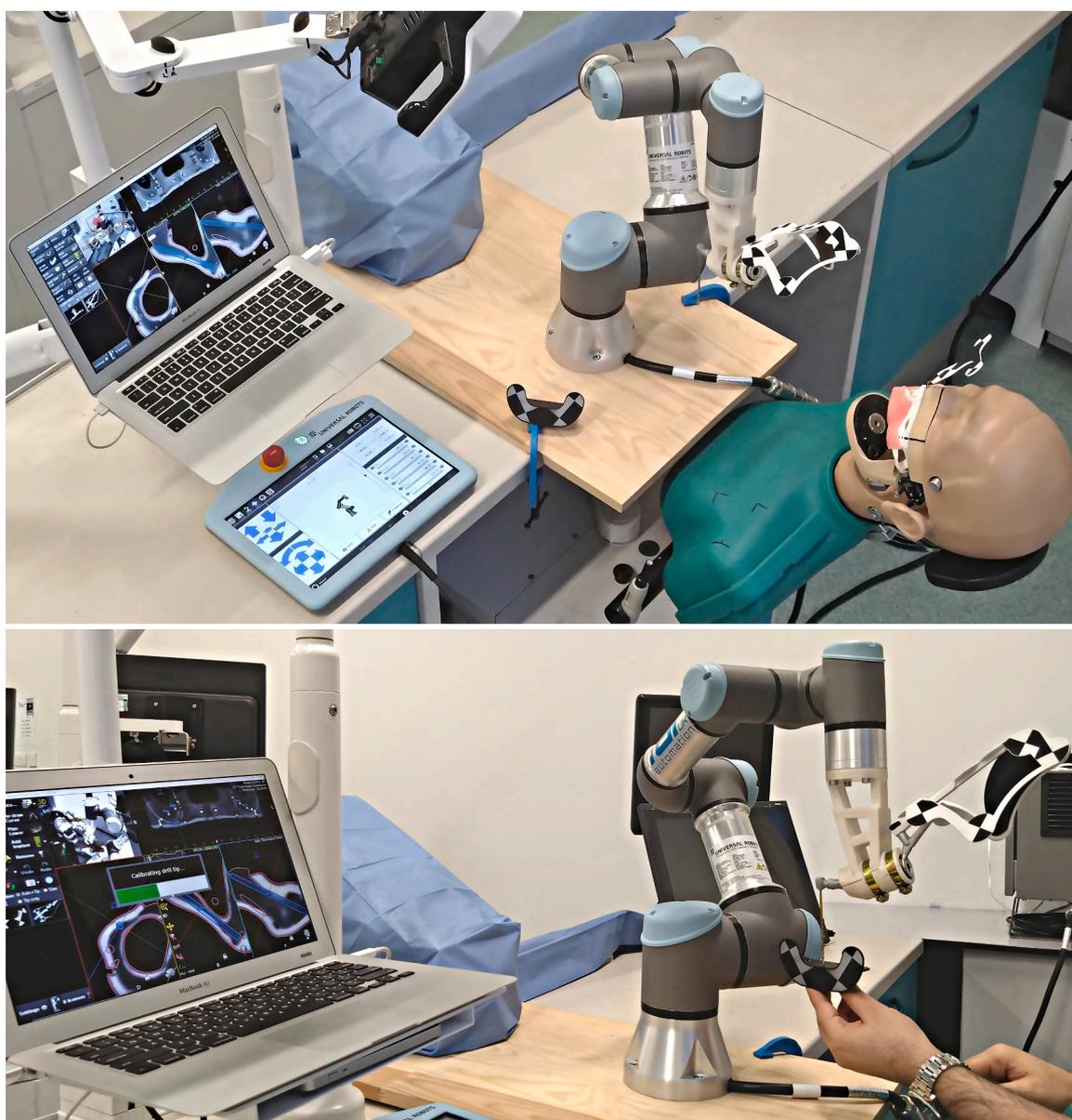
**Fig. 1.** Photographs showing the experimental set-up for the assessment of drill calibration reproducibility. The robotic arm here only serves to fix the spatial relationship of the handpiece tracker and the jaw tracker in relation to the tracking camera through the entire experiment.
