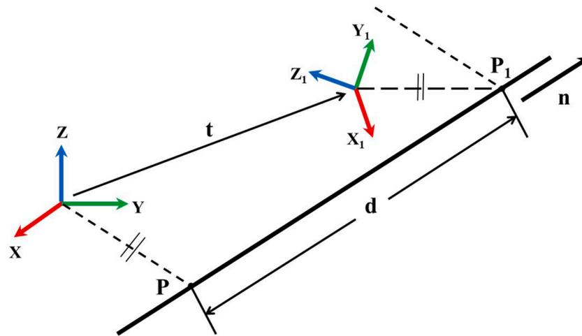
**Fig. 3.** An illustration of the transformation of a point coordinate frame.  $t$  = the transformation movement between the two reference frames;  $XYZ$  represent the original frame;  $X_1Y_1Z_1$  represents the new frame;  $P$  = the original point pre-transformation;  $P_1$  = the transformed point.  $d$  = the distance between the pre- and post-transformed points.  $n$  = the direction vector of point  $P$  transformation (this figure was adapted from Walker et al. [26]).
